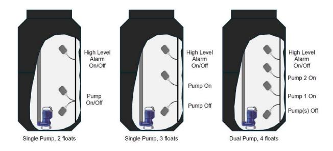
Minimum cable length from attachment pivot point to float head = 100mm
