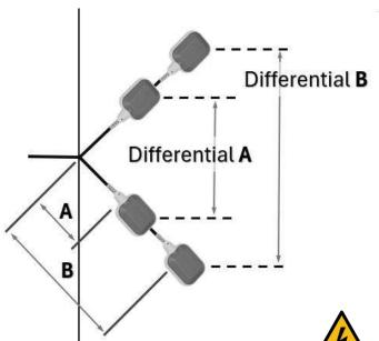
Floats can be supplied as '2 wire' or '3 wire' (allowing either UP or DOWN to be an active switch function). Care should be taken when wiring' 3 wire' floats that the switching is correct
