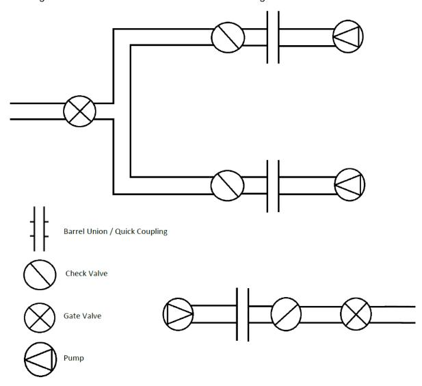
Note: Ball type non return valves should be used in sewage applications.
